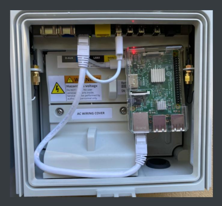
The black port is LAN1, the yellow port is WAN/LAN2! Raspberry powered from USB port 1. Using short cables, plenty of space.
