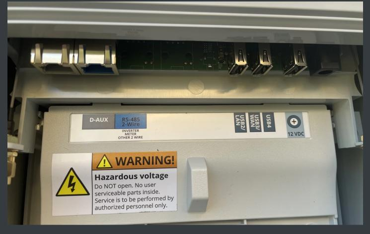
Note that the traditional ethernet ports are no longer there, but there are two USB ports that are also labeled LAN and WAN respectively. Of course, USB does not equal ethernet so the suspicion is that the USB ports can accept ethernet adapters, but so far those that have tried to use ethernet this way have not been successful.
