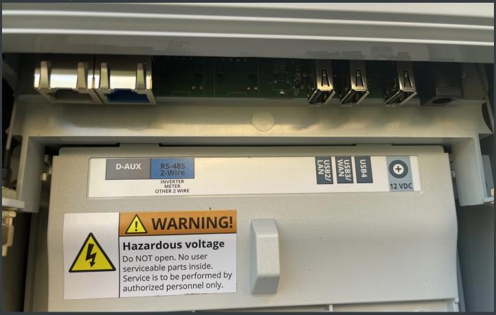
Note that the traditional ethernet ports are no longer there. There are two USB ports that are also labeled LAN and WAN respectively. Of course USB does not equal ethernet so the suspicion is that the USB ports can accept ethernet adapters, but so far those that have tried to use ethernet this way have not been succesful.
