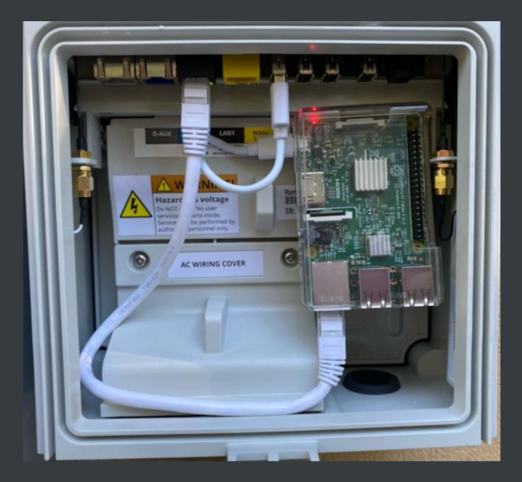
The black port is LAN1, and the yellow port is WAN/LAN2! Raspberry powered from USB port 1. Using short cables, plenty of space.
